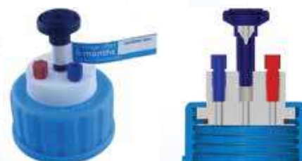
VWR Safety Cap Extracts solvents / mobile phases safely from the bottle or reservoirs without letting the hazardous vapor come out in the lab and prevents unwanted changes in pH of solvent
